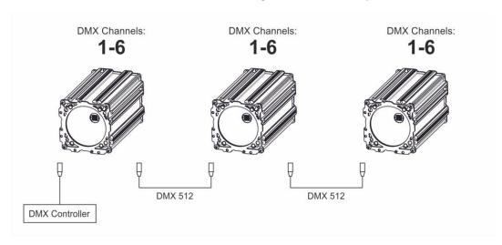
Changing mode is done using a standard DMX controller. Changes can be made by setting the appropriate value in the FUNCTION channel (see DMX channels table). Changing mode is done by setting the appropriate value and waiting 10 seconds.
