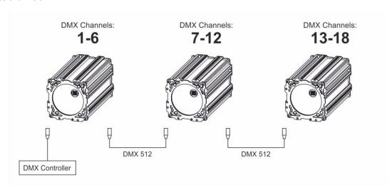
In this way it is possible to connect multiple devices and have independent control of each of them immediately, after turning the power on (without setting the individual DMX addresses using display).
